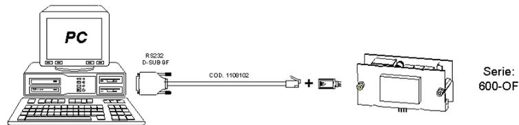
**GF\_eXK-1-1-0: RS232 (PC side)-RS-485 (instrument side)**
