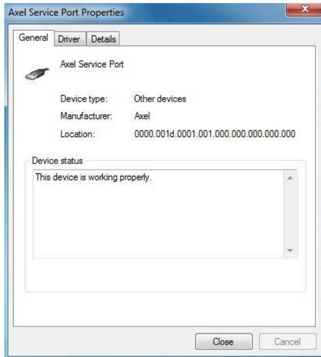
8. Verify in the Device status box the device is working properly; click *Close* for complete the procedure
