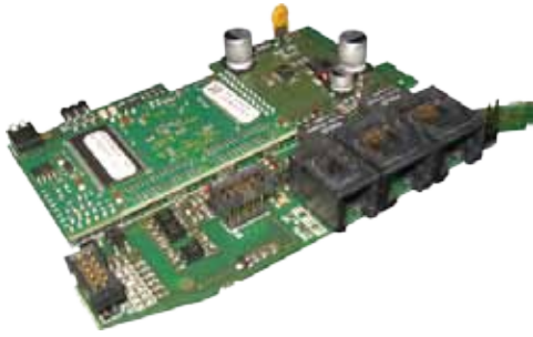
Figure 28 Port2: Modbus RTU / Ethernet IP or Modbus RTU/EtherCAT or Modbus RTU / ProfiNET Interfaces
