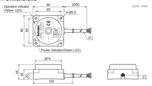
\*\*Cable specification: Ø5, 4 cores(Conductor cross section: 0.3 mm2, Insulator diameter: Ø1.25)
